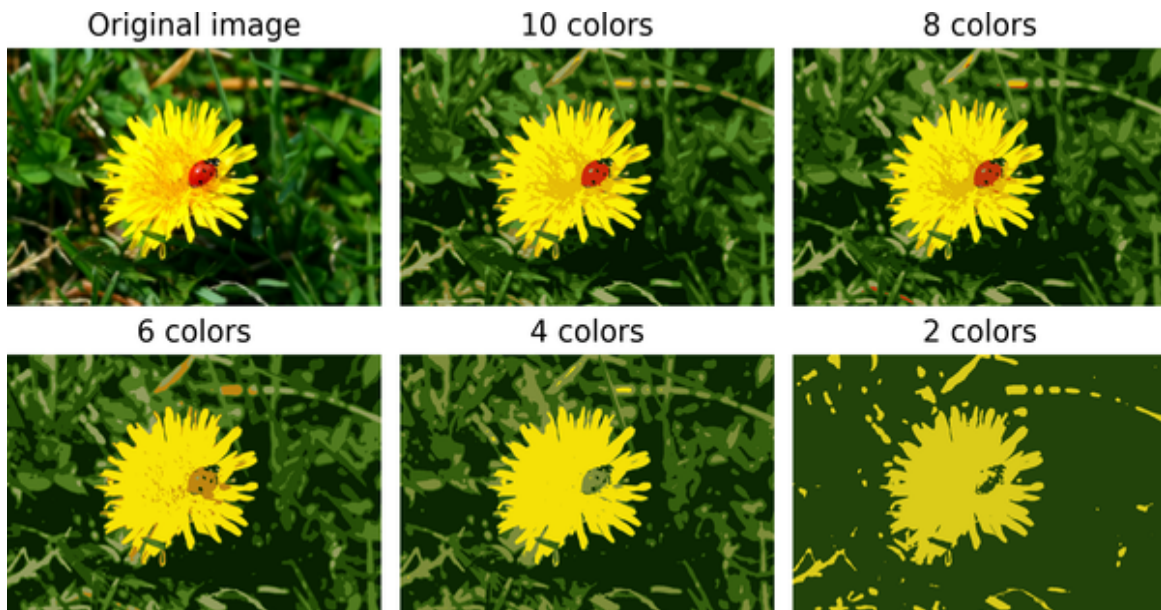
Figure 9-12. Image segmentation using k -means with various numbers of color clusters
